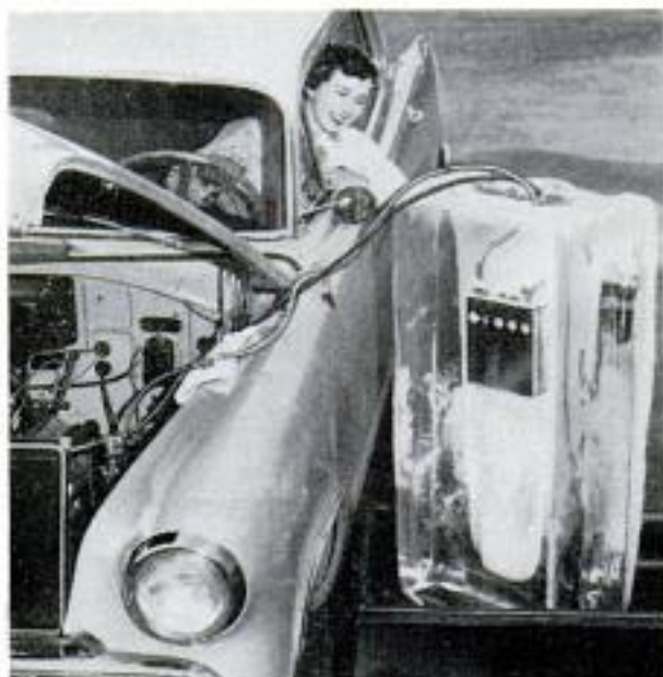
Early nickel-cadmium batteries failed in extreme cold. Sintered-plate type, frozen in ice, starts car quickly
